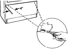
1. Remove access panel by releasing two locking clips with a small, flat-blade screwdriver. The clips are located four inch es in from each side of the access panel. Repeat for other access panel.
